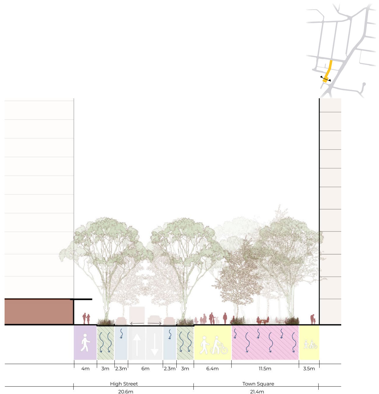
Figure 47. Section - New High Street
